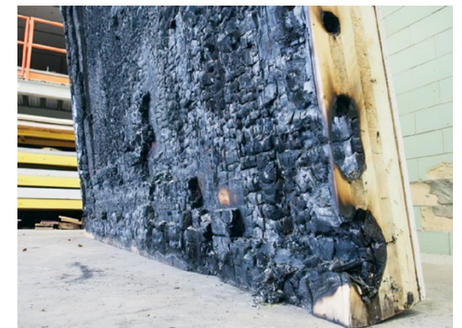
Wall assembly after testing showing the depth of charring on the exposed side. NRC (2014) Fire Endurance of Cross Laminated Timber Floor and Wall Assemblies for Tall Wood Buildings.
