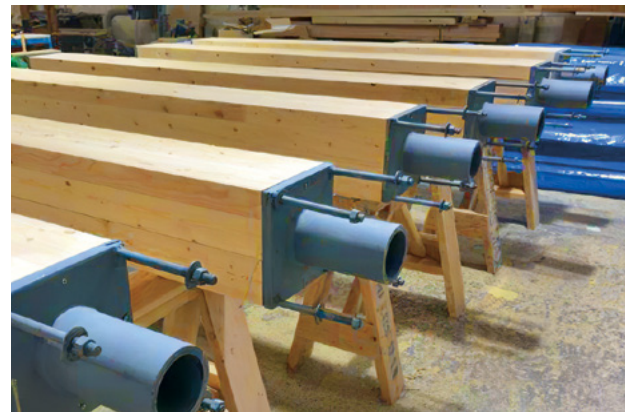
Factory-installed custom steel connectors to be designed by engineer of record or specialty engineer
