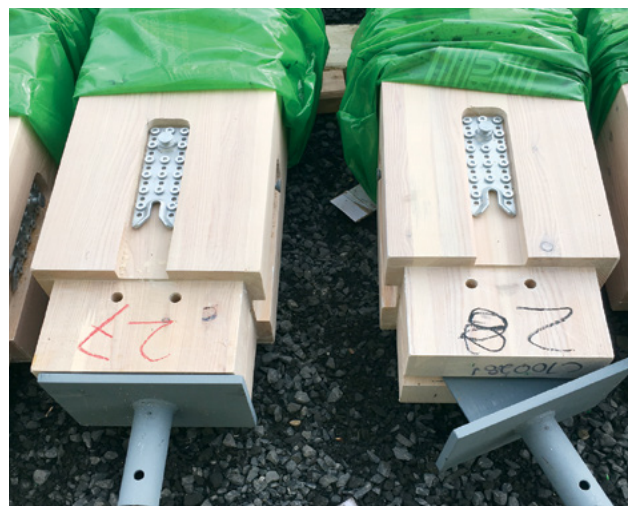
Concealed pre-engineered beam to column connectors
