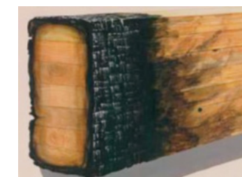
Protective "char layer" maintains structural integrity of interior section.
